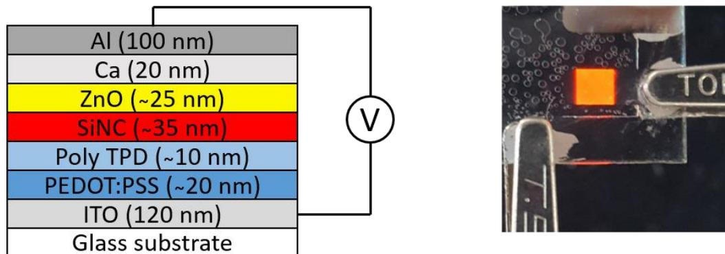
**Figure1:** Used SiNC-LED stack with the target thicknesses of each individual layer and a photo of a working SiNC-LED
